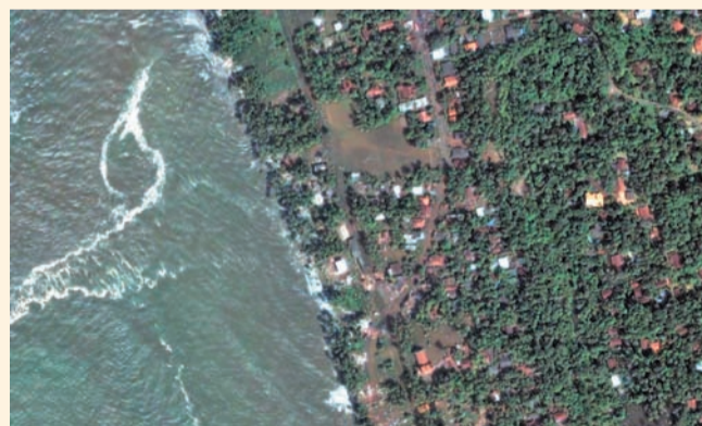
Figure 5: This pattern of high and low water levels is also clearly illustrated in satellite images. In the left figure the original coastline can be seen with a small strip of beach. In the middle figure the tsunami has hit the coast and is penetrating inland. On the left a retreat of the sea is visible now showing a large piece of beach, with the sea tens of meters away from the original coastline.
